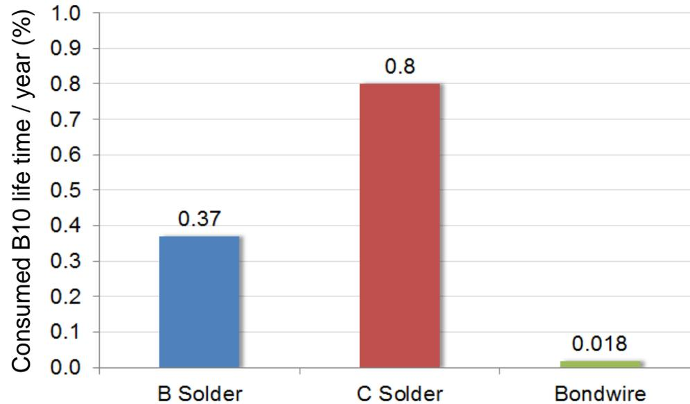
Consumed life time vs. different failure mechanisms.
