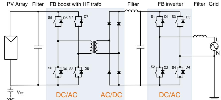
Boosting inverter with HF trafo based on FB boost converter
