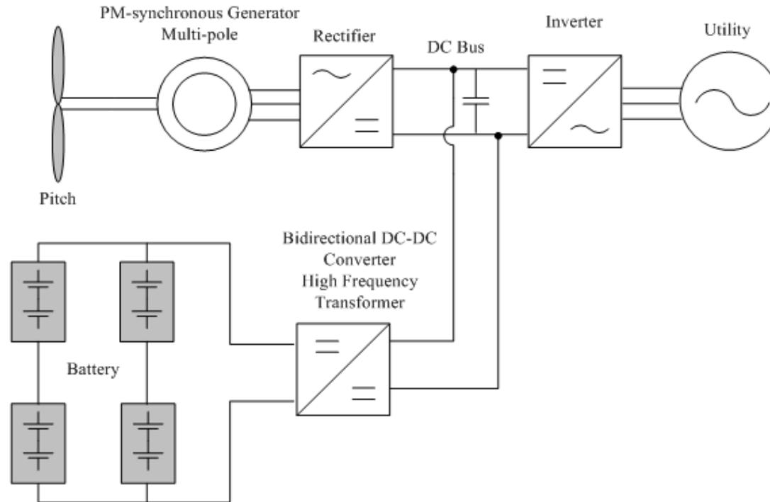
Variable speed wind turbine integrated with a battery storage system
