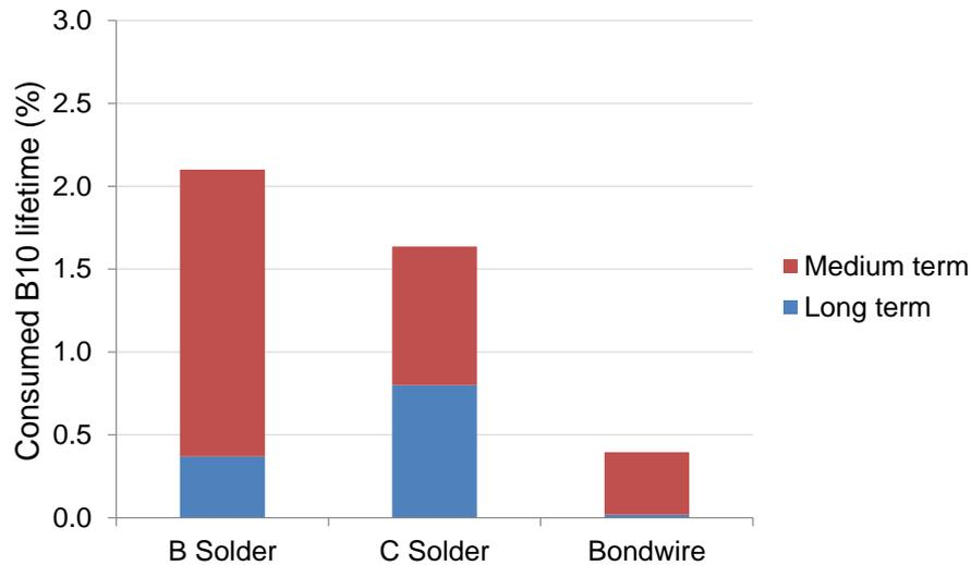
Consumed life time vs. different failure mechanisms.
