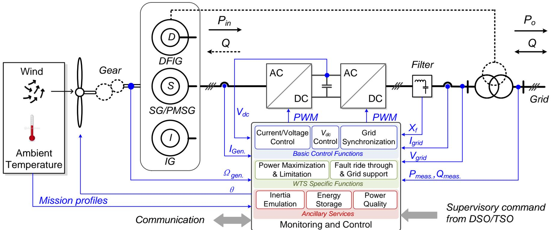
Power has to be controlled by means of the aerodynamic system and has to react based on a set-point given by a dispatched center or locally with the goal to maximize the power production based on the available wind power.
