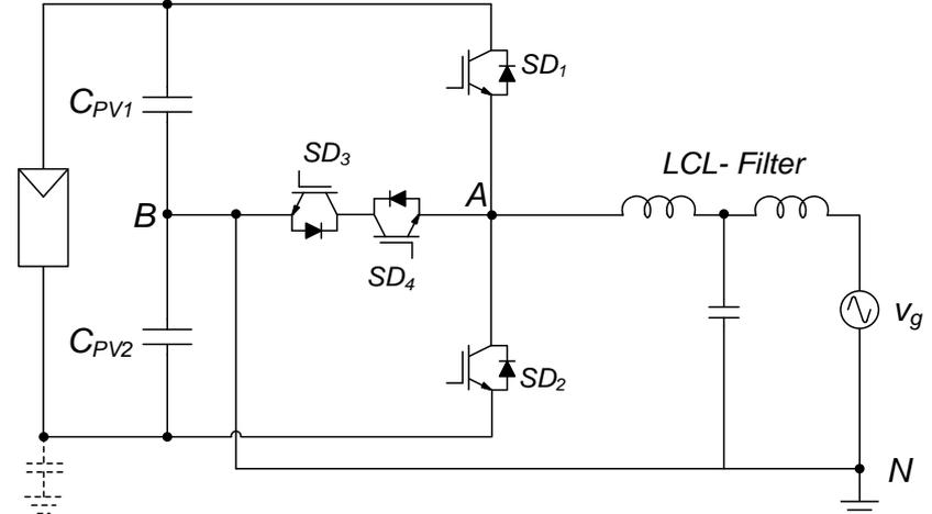
Conergy neutral point clamped inverter
