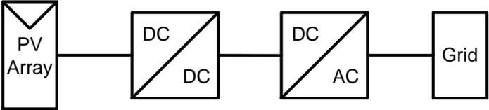
Full Bridge Inverter with Boost Converter
