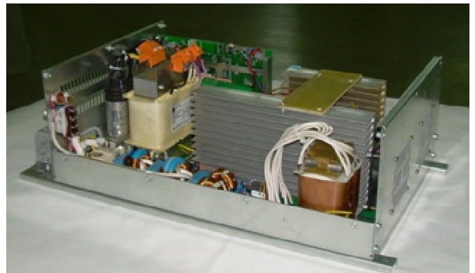
Figure 21. TLBC breadboard with three-phase inverter at output, P_o = 3 kW
