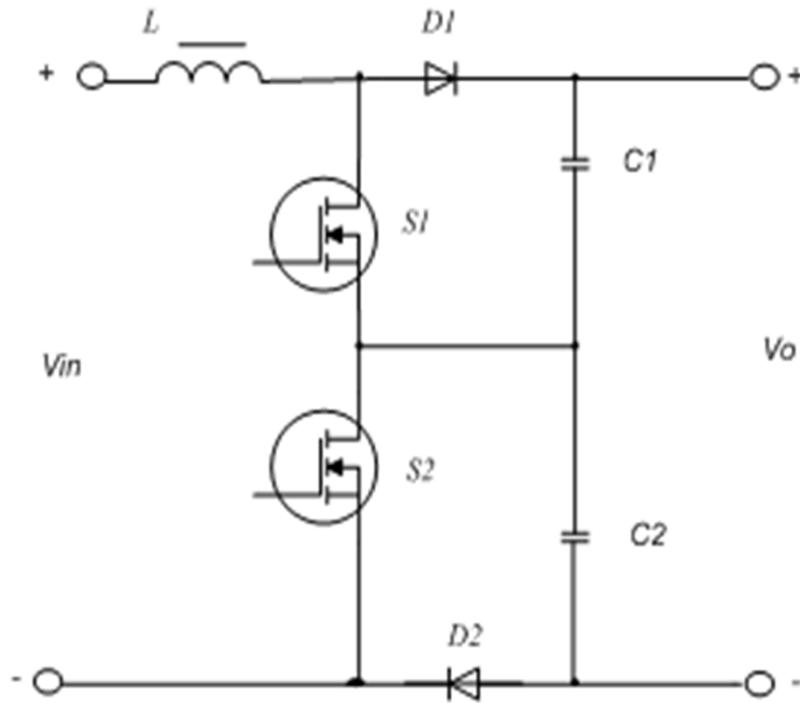
$$V_o = 2V_c = 2V_{in} / (2 - D) \quad \text{TFR for control a)}$$
