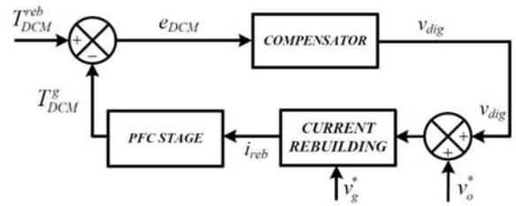
Fig. 5. Block diagram of the DCM time compensation controller.
