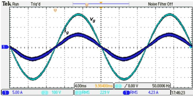
Fig. 10. Experimental results.  $V_g = 229$  V,  $f_u = 50$  Hz,  $THDi = 1.88$  %,  $PF = 0.999$ ,  $P_g = 964.6$  W
