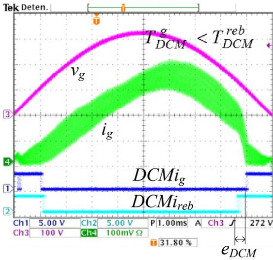
Fig. 8. Real waveforms. Input voltage  $v_g$ , real input current  $i_g$ , waveforms and digital for the cases: above  $e_{DCM} < 0$  and below  $e_{DCM} > 0$
