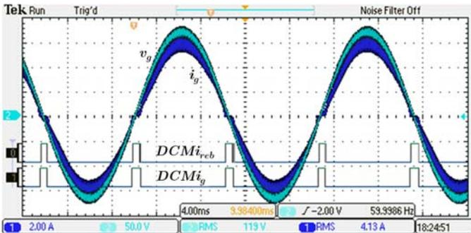
Fig. 21. Experimental results.  $V_g = 119$  V,  $f_u = 60$  Hz,  $THDi = 2.15$  %,  $PF = 0.998$ ,  $P_g = 491.3$  W
