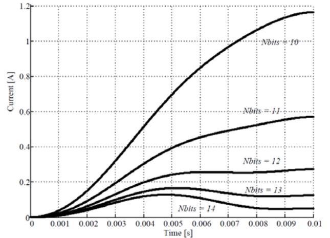
Fig. 6. Current estimation error resolution for different bits of resolution
