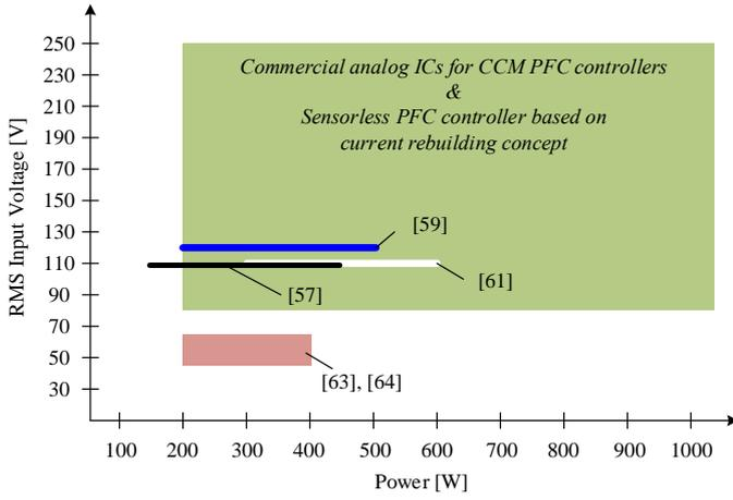
Fig. 3. Input voltage and power range of the recent works in sensorless PFC controllers.
