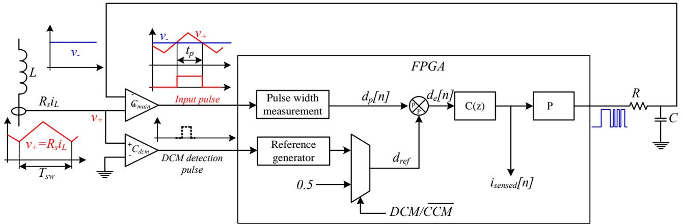
Fig. 1. Average current sensor scheme.
