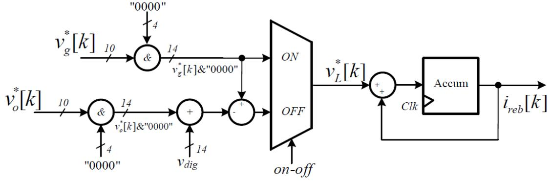
Fig. 7. Current estimator hardware implementation with higher resolution.
