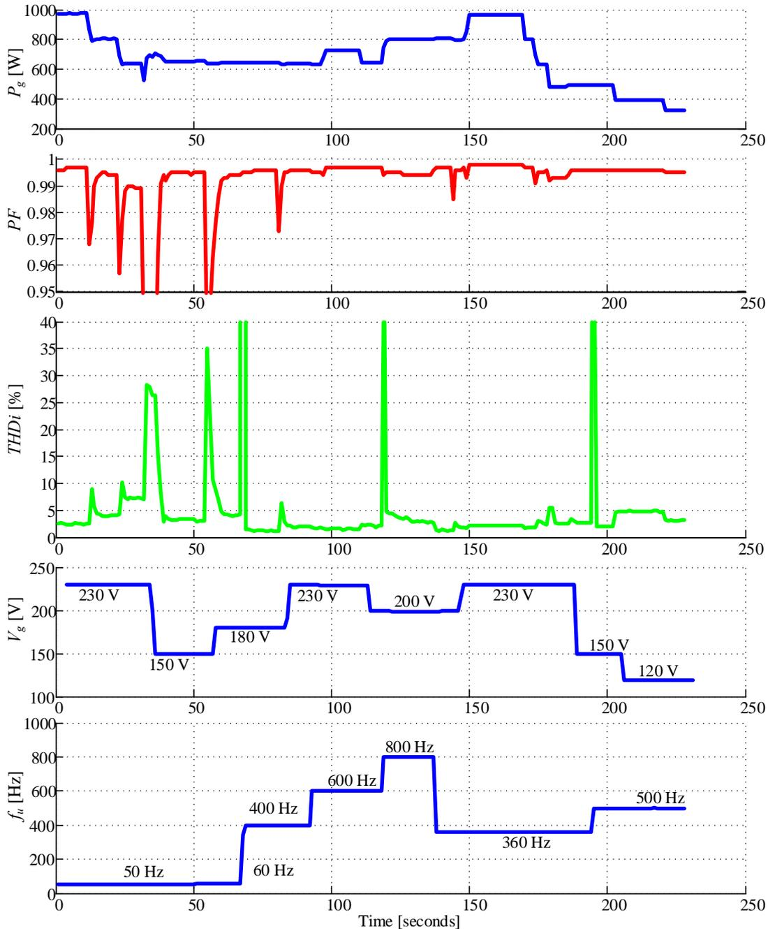
Fig. 9. Time evolution of the different electrical variables with  $V_o = 400 V_{dc}$ ,  $f_{sw} = 96 \text{ kHz}$
