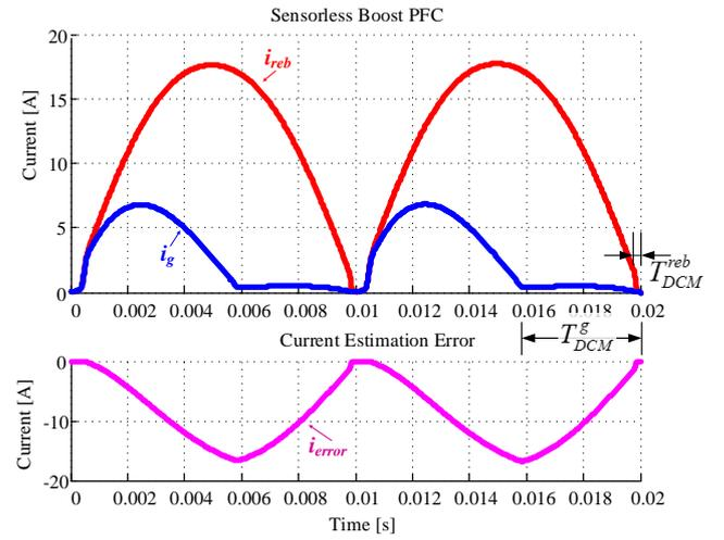
Fig. 4. Current waveforms under a current estimation error situation.
