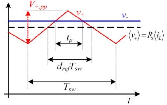
Figure 2. Operating waveforms of the average current sensor.
