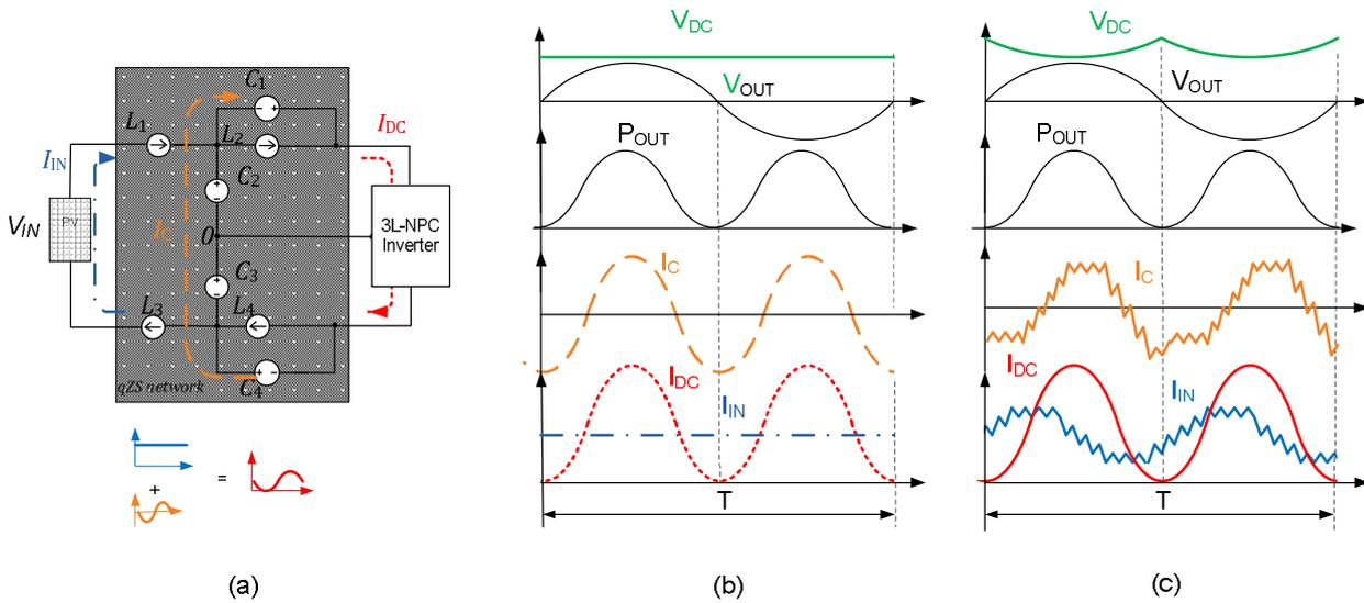
Fig. 3. Equivalent scheme and diagrams in the CCM.
