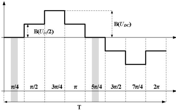
Fig. 4. Output voltage waveform of the traditional shoot-through PWM for the 3L-NPC qZSI.
