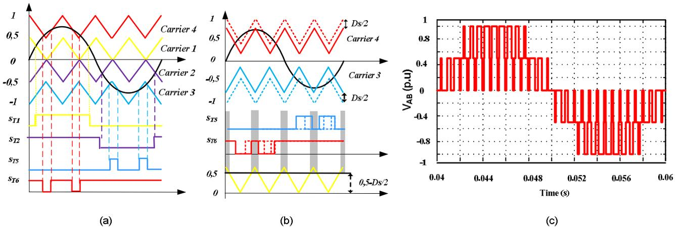
Fig. 5. Sketch of the proposed modulation technique with uniformly distributed shoot-through states and constant width.
