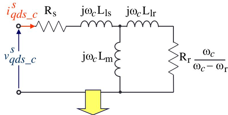
High frequency equivalent circuit
