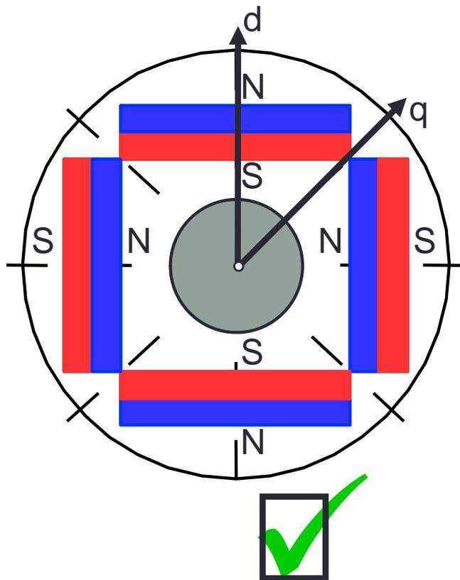
Radial flux, surface permanent magnet machines
