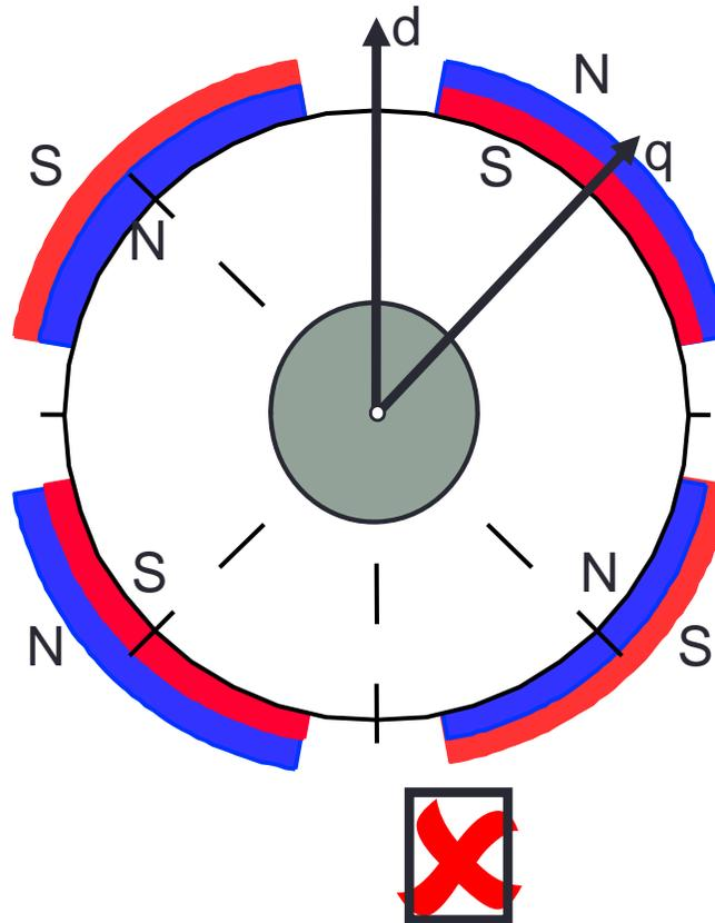
Tangential flux, interior permanent magnet machines
