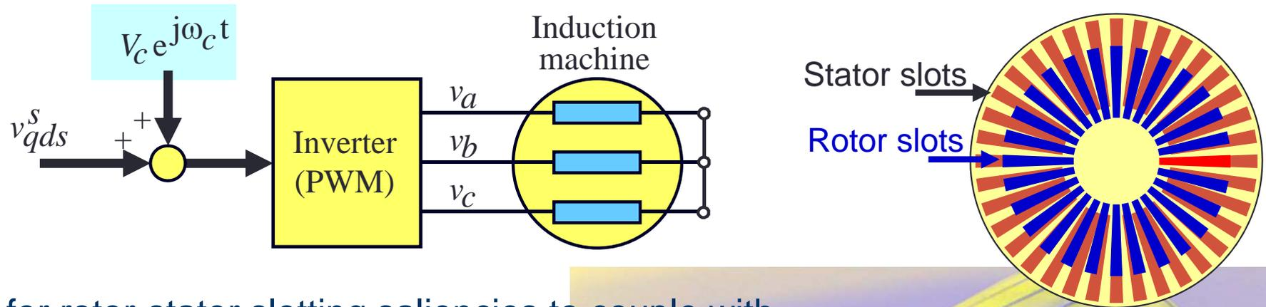
Requirement for rotor-stator slotting saliencies to couple with the stator windings and produce measurable signals:
