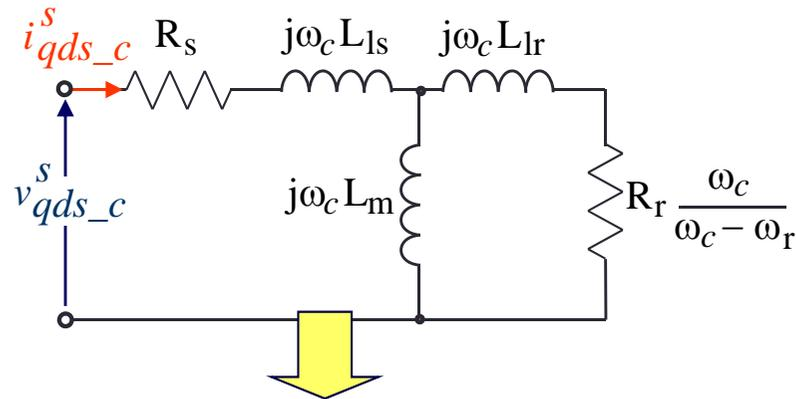
High frequency equivalent circuit
