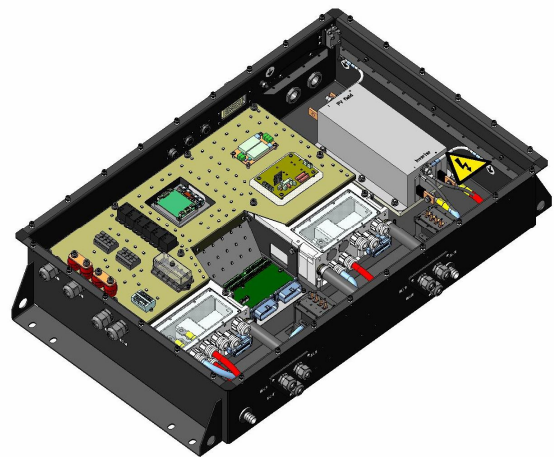
Figure 6. SKAI2-based PEB for the TEES of a hybrid bus.
